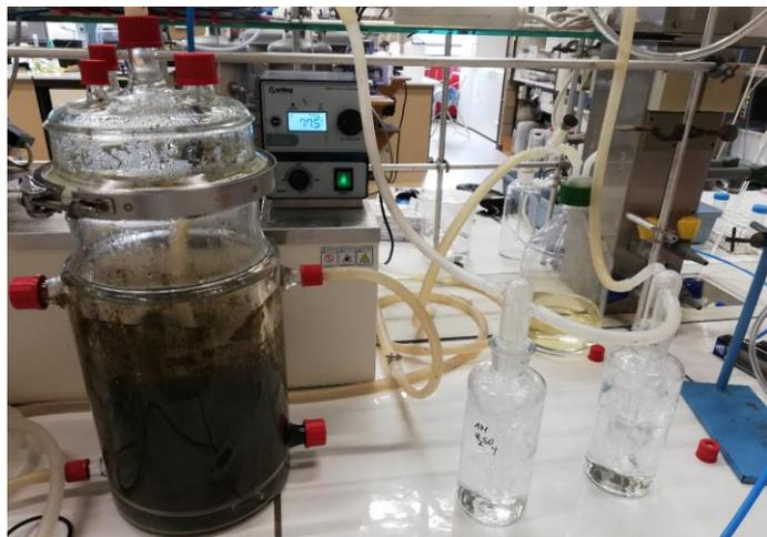
Figure 1: stripping-scrubbing set-up
