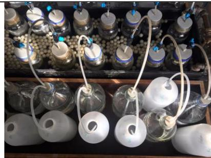
Figure 1: BMP assay set-up, top view
